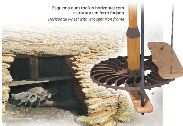
Rodízio do moinho de Estanislau The horizontal wheel of Stanislaus's water mill
